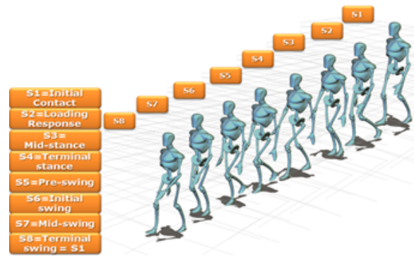
Figure 3: Internal gait phases of human normal gait cycle used in the MOBOT project to extract gait parameters and analyse walking impairments.
