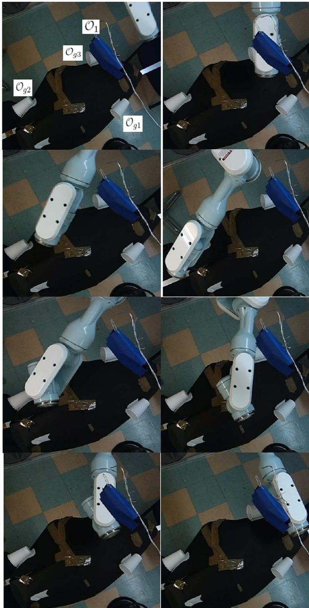
**Fig. 9** Experimental Set-up. Top view of experimental. The robot manipulator is moving towards the (black) surface, avoiding blue obstacles. The end-effector reaches its destination configuration (second right picture). The white cups on the surface are being avoided during the tracking phase, that follows the stabilization to the destination configuration.
