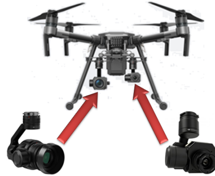
Fig. 9: Intergraded drone dji MATRICE 210 with dual downward gimbals, optical camera dji ZENMUSE X5S (left) and thermal dji ZENMUSE XT (right).
