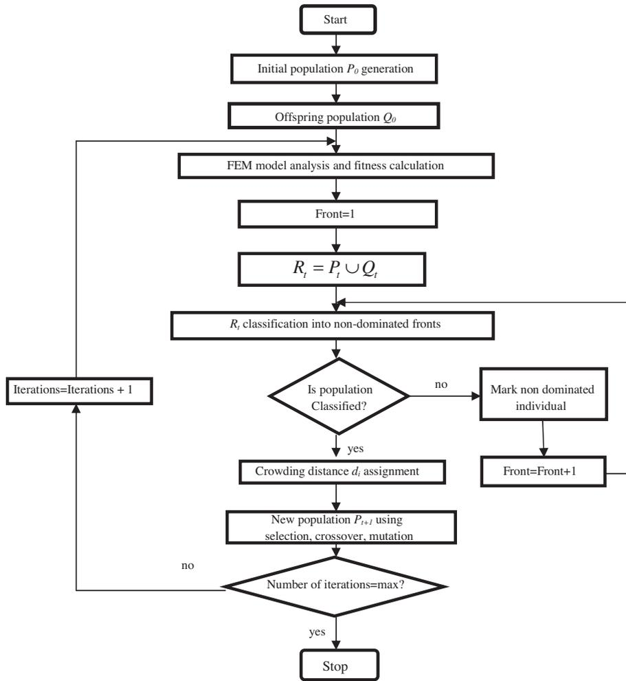
Fig. 3. Schematic flowchart of the NSGA-II as implemented.
