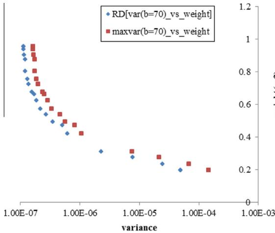
**Fig. 7.** Pareto front for classical RDO for a given field with  $b = 70$  and total weight as objective functions and maximum possible variance for the selected designs. Variance axis in logarithmic scale.
