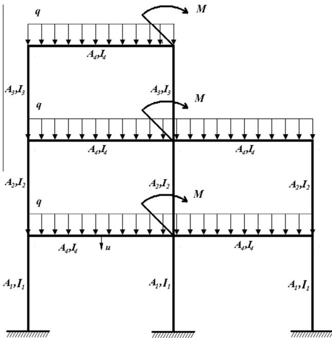
Fig. 1. Geometry and loading of the fixed–fixed frame discretized with 60 beam elements.
