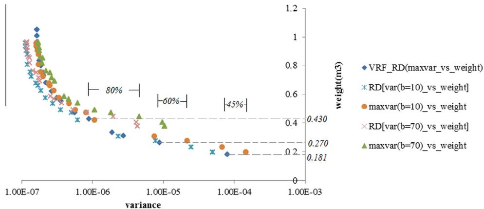
**Fig. 8.** Pareto fronts for classical RDO with variability response for a given field with  $b = 10, 70$  and total weight as objective functions with respective maximum possible variances for the selected designs and Pareto front with *VRF* and total weight as objective functions. Variance axis in logarithmic scale.
