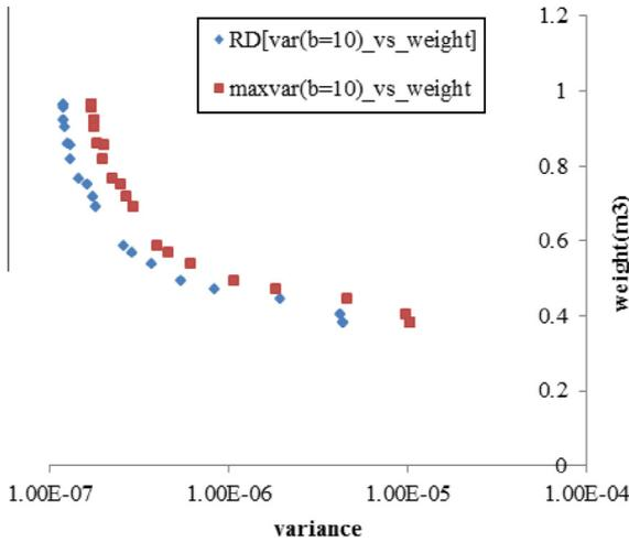
Fig. 5. Pareto front for classical RDO for a given field with  $b = 10$  and total weight as objective functions and maximum possible variance for the selected designs. Variance axis in logarithmic scale.
