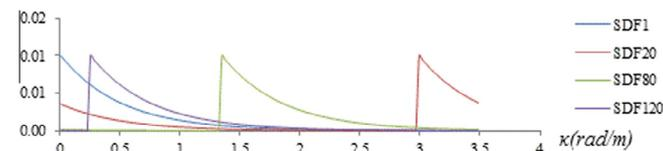
Fig. 2. Plots of different spectral density functions of the  $S_p$  family for a discretization of 128 steps in the frequency domain.
