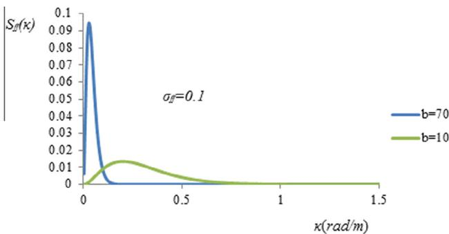
Fig. 4. Spectral density functions for stochastic field  $f(\mathbf{x})$  standard deviation  $\sigma_{ff} = 0.1$  for two different values of the correlation length parameter.
