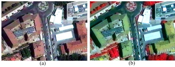
Fig. 7 Sample of G1 training image. (a) Natural RGB composite, (b) Pseudo-color composite containing NIR (Red color: NIR band, green color: RED band, blue color: GREEN band)
