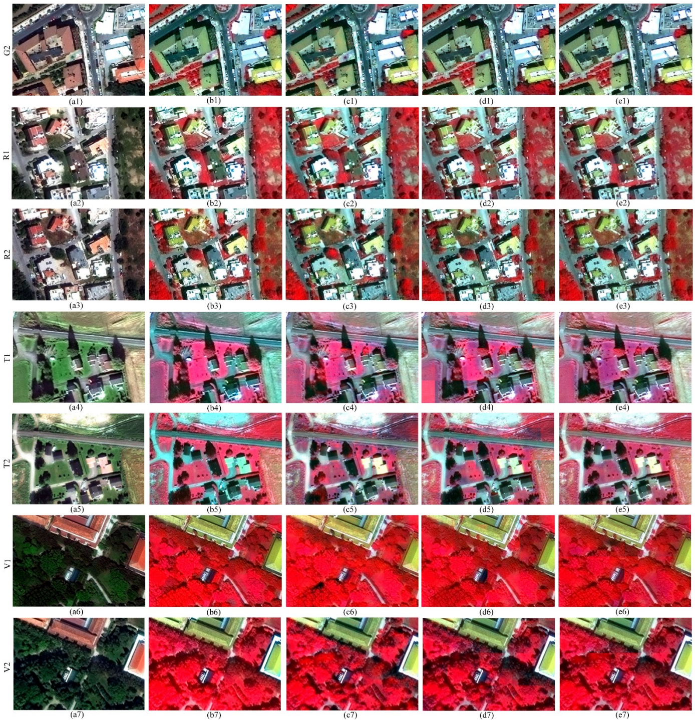
Fig. 6. Samples of pseudo-color composites of the NIR predictions in the paired ITIT (first stage). Red color is assigned to the NIR band, green color to the RED band, and blue color to the GREEN band. (a1-a7) Natural RGB composite, (b1-b7) Ground-truth, (c1-c7) Pix2Pix, (d1-d7) AWAN, (e1-e7) MST++.
