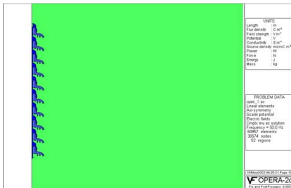
Figure 3: The Finite Element Model of the simulated insulator string.
