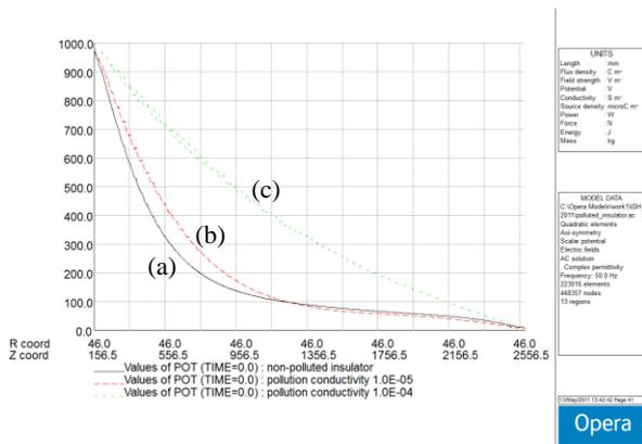
**Figure 7:** The potential distribution on a vertical line across the edges of the weathersheds ( $R=46\text{mm}$ ) calculated with the steady state ac solver for
