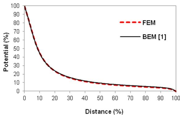
**Figure 2:** The potential distribution along the insulation distance at the centre line of the rod (R=0mm).
