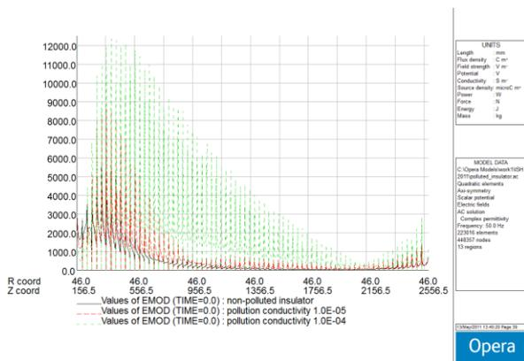
**Figure 8:** The electric field distribution on a vertical line across the edges of the weathersheds ( $R=46\text{mm}$ ) calculated with the steady state ac solver for
