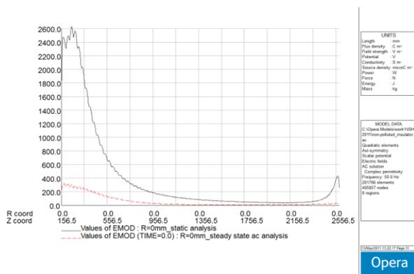
**Figure 5:** The electric field distribution along the centre line of the rod (R=0mm) calculated with the static and the steady state ac solver.
