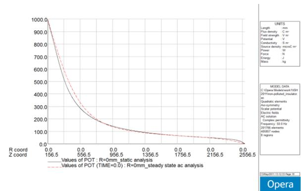
**Figure 3:** The potential distribution along the centre line of the rod (R=0mm) calculated with the static and the steady state ac solver.
