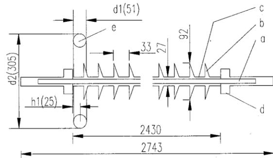
**Figure 1:** Simplified geometry and dimensions of the nonceramic insulators to be modeled: (a) fiberglass rod (b) polymeric material weathersheds (c) polymeric material sheath (d) metal end fitting and (e) grading ring [1].
