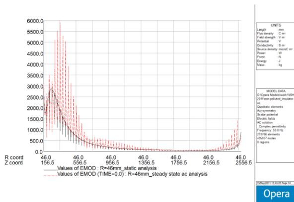
**Figure 6:** The electric field distribution on a vertical line across the edges of the weathersheds (R=46mm) calculated with the static and the steady state ac solver.
