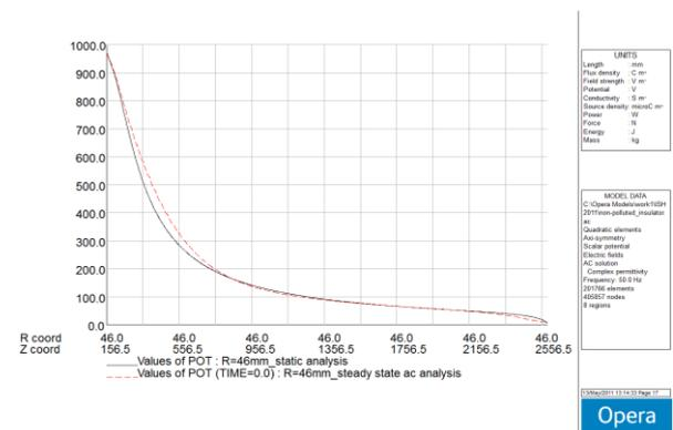
**Figure 4:** The potential distribution on a vertical line across the edges of the weathersheds
