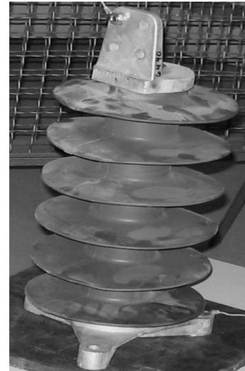
**Fig.2 Examined polymeric housing gapless metal oxide surge arrester**
