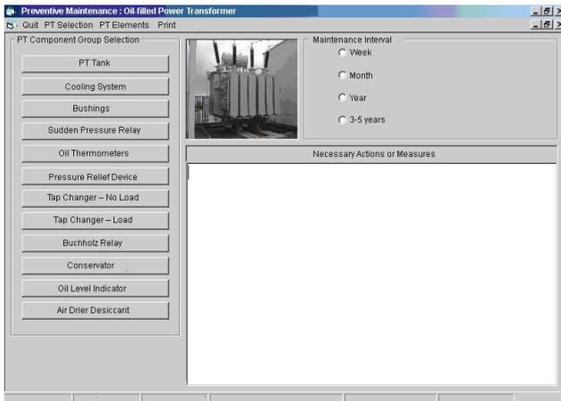
**Figure 2.** PTME sample screen showing PT component groups and maintenance intervals to be selected.
