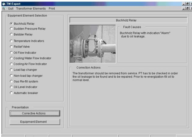
**Figure 7.** PTME Corrective Maintenance sample screen containing suggestions about the required remedial measures
