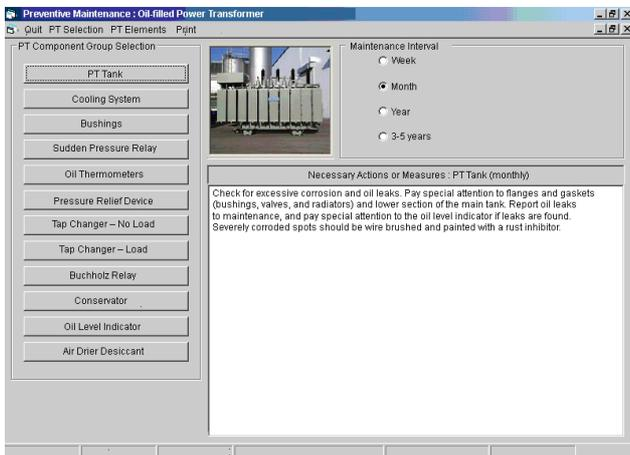
**Figure 3.** PTME sample screen showing proposed PT tank preventive maintenance actions on monthly basis.
