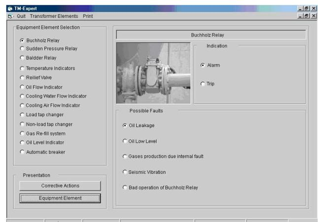
**Figure 6.** PTME Corrective Maintenance sample screen in the case of an activated alarm of a PT Buchhotlz relay, which implies oil leakage.
