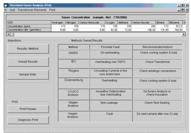
**Figure 5.** PTME predictive maintenance overall results of dissolved gas analysis in a PT, showing possible fault determination and recommended actions.
