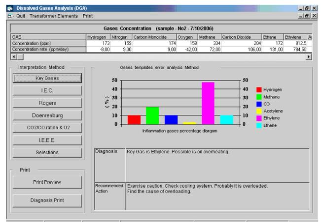
**Figure 4.** PTME sample screen showing dissolved gas test analysis results according to selected interpretation method (Key Gases).
