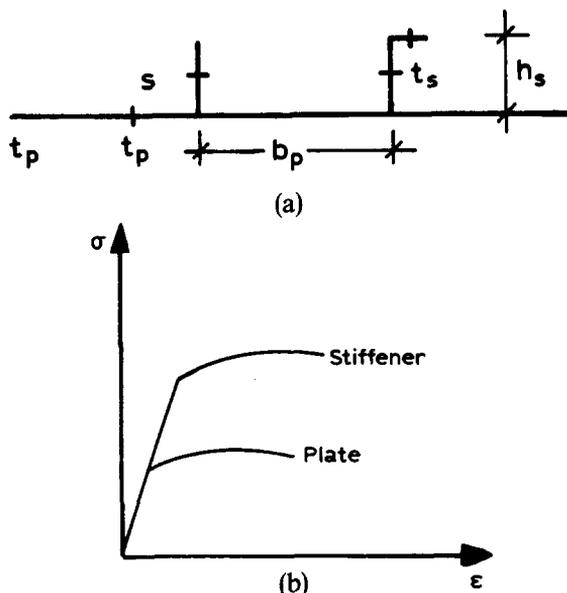
Fig. 2. Notation for and behaviour of, stiffened plates.
