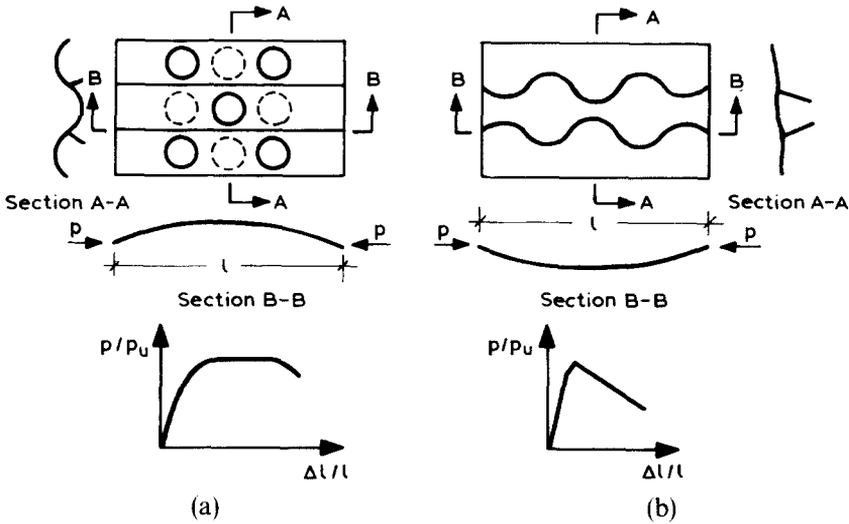
Fig. 1. Failure modes of axially compressed, stiffened plates. (a) Plate failure; (b) Stiffener failure.
