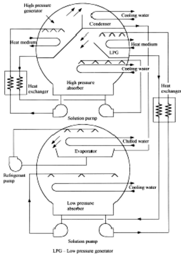
Fig. 5. Two stage absorption chiller (Ref. [31])
