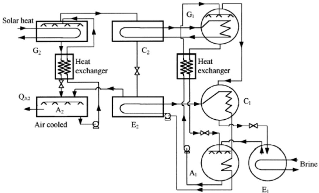
Fig. 7. Dual-cycle block diagram (Ref. [31])
