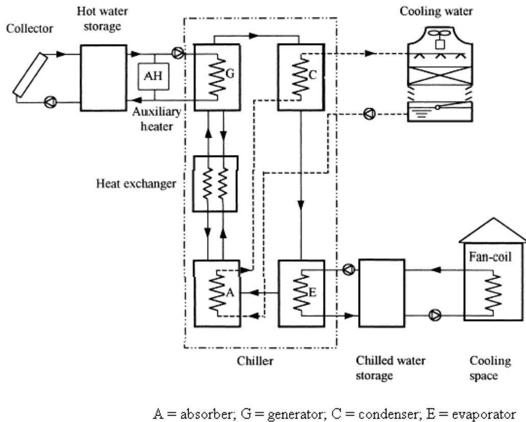
Fig. 1. Solar powered single-effect air-conditioning system (Ref. [31])
