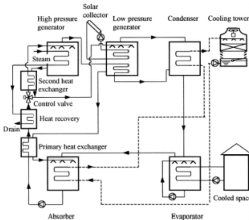
Fig. 4. Single/Double Effect Convertible Absorption Cooling System (Ref. [31])
