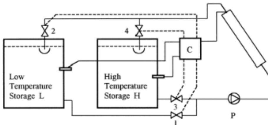
Fig. 3. Schematic diagram of a dual storage system (Ref. [31])
