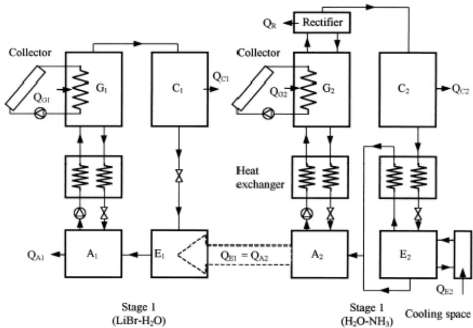
Fig. 6. Two-stage dual fluid solar absorption cycle (Ref. [31])
