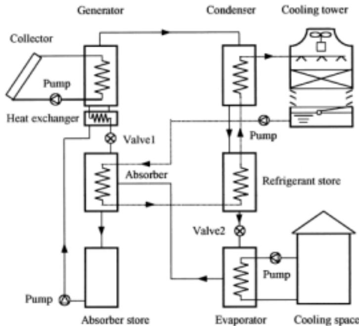
Fig. 2. Solar cooling system with refrigerant storage (Ref. [31])
