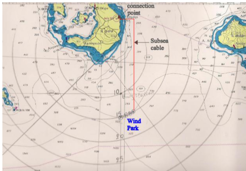
Fig. 8. Spatial design of the wind turbines indicating wind turbines, subsea cable and onshore connection point, using the map of the Navy Hydrographic Service.
