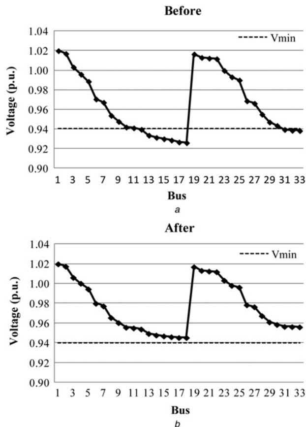
Fig. 6 Voltage variations at each node of the 33-bus distribution system before and after DG placement for Scenario 1
