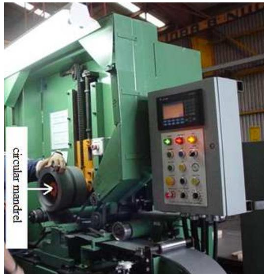
Fig.1. Manufacturing of CWC on circular mandrel.
