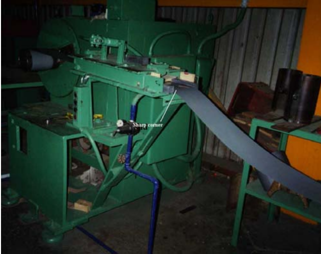
Figure 2. Stress introduced when the steel roll is hauled to manufacture the core.
