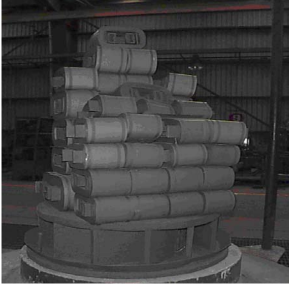
Figure 1. Arrangement of the core pile after the annealing process. Four superior cores of this pile are fallen due to incorrect movement of the furnace cover and these cores should be re-annealed.
