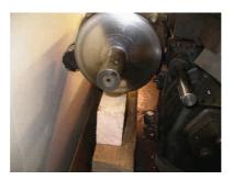
Chock up the motor and remove its four fixing screws. Remove the motor speed lever and release the two caps screws from the headstock cover. Now, lift off as one unit the motor, headstock cover, and the power input cable. (It's useful if you have help to carry the unit (headstock cover, motor, and input cable) to and from the lathe, although I managed it alone).
