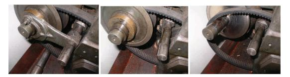
First remove the end bracket by removing just two screws. Next slacken the cap screw holding the LH fork to the shaft and slide the fork off. You can then slide off the LH pulley face.
