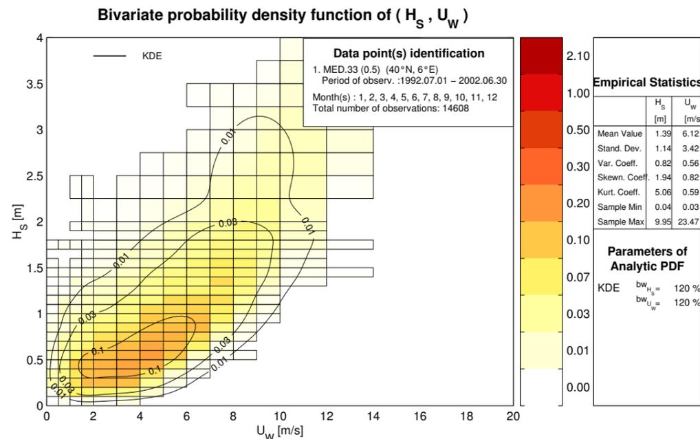
Figure 16 - Joint wind-wave statistics for datapoint (6E,40N)
