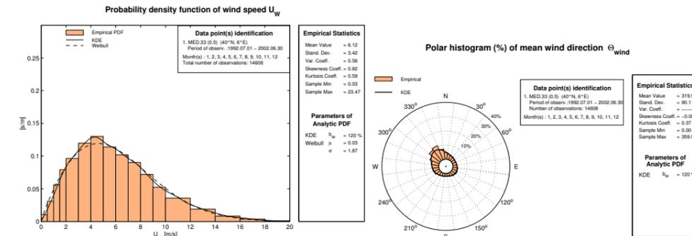
Figure 10 - Examples of wind statistics for datapoint (6E,40N).
