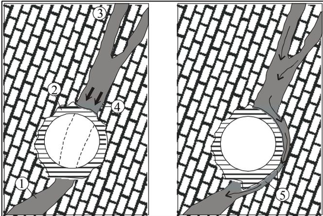
Figure 15: Crossing a big karst conduit by tunnelling (Milanović, 2000). 1. Karst, 2. Tunnel, 3. Water level in the channel, 4. Lining under concentrated pressure, 5. Drainage around the tunnel pipe.
