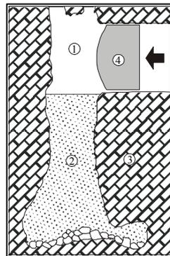
Figure 17: Cavern treatment by concrete filling for a TBM drive (Milanović, 2000). 1. Cavern; 2. Part of cavern filled by concrete; 3. Limestone; 4. TBM.
