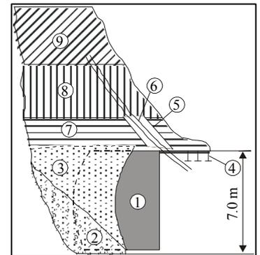
Figure 19: Filling of a cavern from inside the tunnel (Milanović, 2000). 1. TBM; 2. Cave clayey deposits; 3. Inert material – sand; 4. Tunnel support; 5. Shaft; 6. Pipe connected with concrete pump; 7, 8, 9. Stages of concreting.
