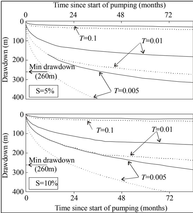
Figure 9: Predicted evolution with time of the average drawdown at the periphery of the mines, for various values of the transmissivity (T) of the aquifer. Pumping intensities: 10.000 m<sup>3</sup>/h (continuous line), and 15.000 m<sup>3</sup>/h (dotted line). Storativity: 5% (upper diagram), 10% (lower diagram).
