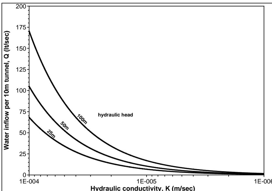
Figure 1: Estimation of water inflow in a 10 m diameter tunnel for steady flow condition. This graph can be applied in the inundation zone of a limestone aquifer for estimating maximum values before transient flow is established and in sections between two main karstic conduits. It does not apply to discharges through the conduits themselves. These conduits may recharge their fractured-jointed limestone environment simulating steady flow conditions.
