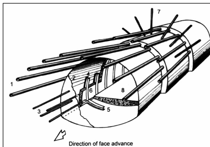
Figure 14: Full face excavation through weak ground under the protection of a forepole umbrella. The final concrete lining is not included in this figure (Hoek, 2000). The method can be applied in cases of large karstic caverns or large chimneys filled with cohesive soil under substantial load. Note that it is not always necessary to implement all the components shown in this figure.
