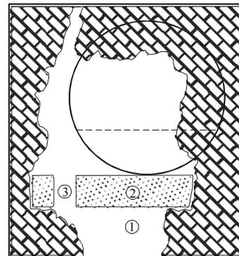
Figure 18: Cavern rehabilitation by bridging for a TBM drive (Milanović, 2000). 1. Cavern; 2. Concrete slab; 3. Aeration – drainage opening.
