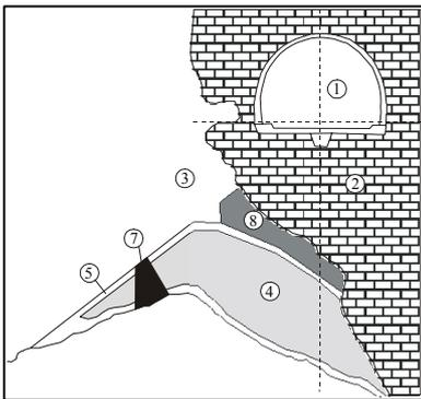
Figure 16: Driving the tunnel over a big karstic cavern. Longitudinal (a) and perpendicular (b) cross-sections (from Hudec et al, 1980). 1. Tunnel, 2. Limestone, 3. Cavern, 4. Fill – aggregate, 5. Fill – reinforced with cement, 6. Stone wall, 7. Retaining wall (reinforced fill), 8. Concrete, 9. Tunnell floor.
