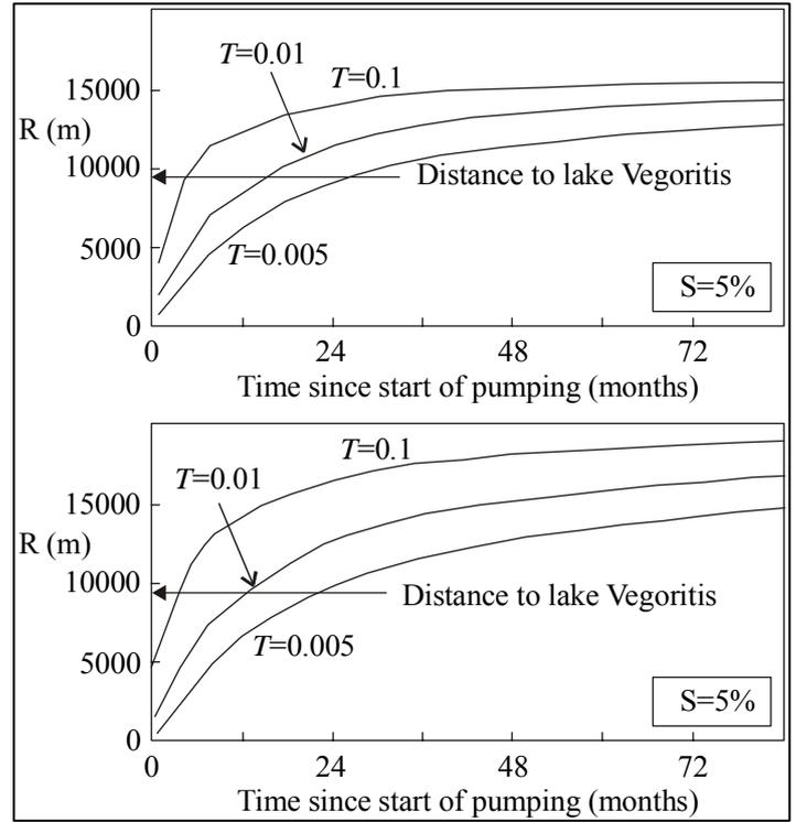
Figure 10: Predicted evolution with time of the average radius of dewatering (defined as the distance at which drawdown is 0.5 m), for various values of the transmissivity (T). Storativity: 5%. Pumping intensities: 10.000 m<sup>3</sup>/h (continuous line: upper diagram) and 15.000 m<sup>3</sup>/h (dotted line: lower diagram).
