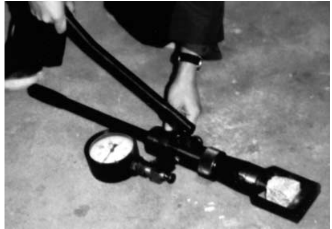
Fig. 3 “Portable” point load test device for use in the field
