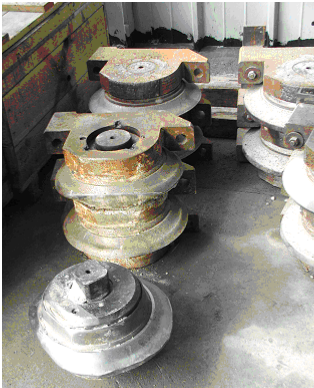
Figure 11: Wear of the disk cutter bearings and bearing mounts. Disks that do not rotate freely wear asymmetrically while freely rotating disks are abraded as shown in Figure 10.
