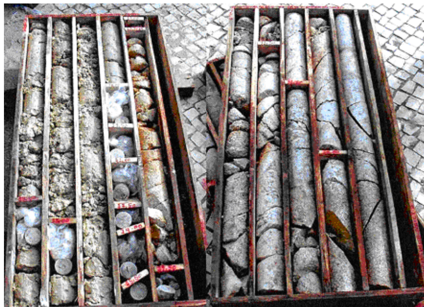
Figure 3: Appearance of different degrees of weathering in granite in a core recovered from a site investigation borehole on the tunnel alignment. Note that the weathered granite in the left box is at a depth of about 24m under the sound granite of the right box. This must therefore correspond to a huge boulder (core).
