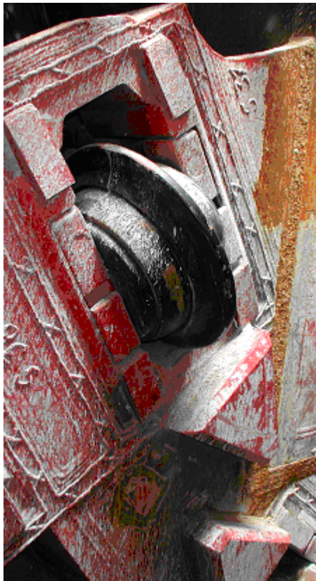
Figure 12: Addition of deflector wedges ahead of disk cutters helped to deflect paste from the bearing assembly.
