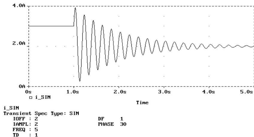
The SIN waveform is for transient analysis only. It does not have any effect on AC analysis. To give a value to a current during AC analysis, use an AC specification, such as:
