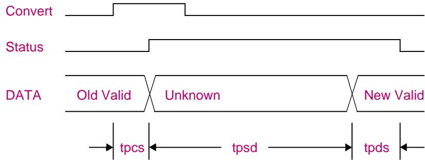
DATA refers to both the data and over-range signals. The Convert pulse can be any width, including zero. If the propagation delay between the rising edge of the Convert signal and the Status signal (tpsd) is zero, the data and over-range do not go to unknown but directly to the new value. There is a resistive load from <ref node> to <gnd node>, and from <in node> to <gnd node>, of 1/GMIN.
