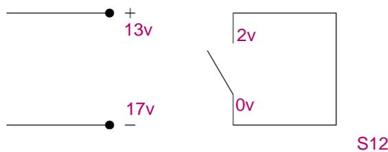
**Comments** The resistance between the <(+) switch node> and <(-) switch node> depends on the voltage between the <(+) controlling node> and <(-) controlling node>. The resistance varies continuously between the **RON** and **ROFF** model parameters.
