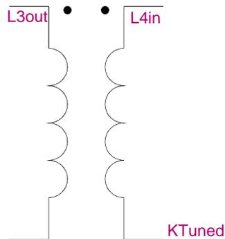
This device can be used to define coupling between inductors (transformers) or between transmission lines. This device also refers to a nonlinear magnetic core (CORE) model to include magnetic hysteresis effects in the behavior of a single inductor (winding), or in multiple coupled windings.
