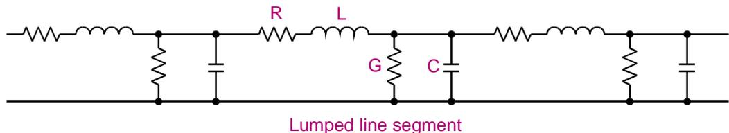
This method requires that there is enough lumps to adequately represent the distributed character of the line, and this often results in the need for a large netlist and correspondingly long simulation times. The method also produces spurious oscillations near the natural frequencies of the lumped elements.
