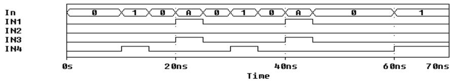
**Five** The fifth example illustrates the use of the INCR BY command used to increment the value of the 16 bit bus:
