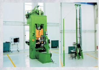
A ball drop forming rig for contour forming.
