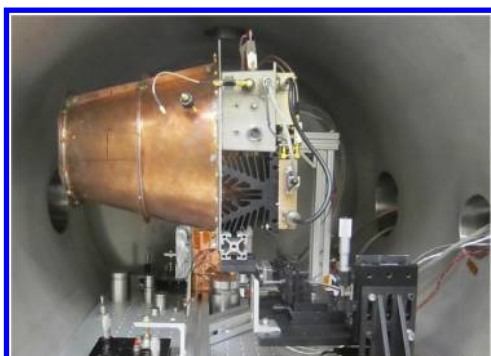
Fig. 14 Forward thrust mounting configuration (heat sink is black finned item between test article and amplifier).
