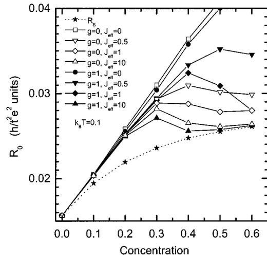
FIG. 1. Resistance as a function of magnetic particle concentration.
