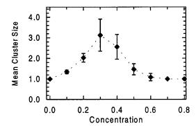
FIG. 9. Variation of the mean cluster size with concentration of magnetic particles. Error bars indicate the dispersion of cluster sizes at each concentration. The infinite (percolation) cluster is not included in the statistics.
