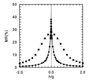
FIG. 12. Field dependence of anhysteretic magnetoresistance of a dipolar sample (squares) and a noninteracting sample (circles). Parameters: p = 30% (Co<sub>16</sub>Cu<sub>84</sub>) and T = 82 K. Coalescence is allowed in both samples.
