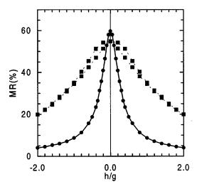
FIG. 4. Field dependence of hysteretic magnetoresistance for a dipolar sample (squares) and for a noninteracting sample (circles). Parameters: p = 30% (Co<sub>16</sub>Cu<sub>84</sub>) and T = 82 K. Monodisperse samples.
