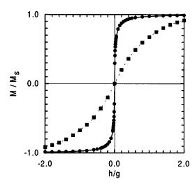
FIG. 11. Anhysteretic magnetization curve for a dipolar system (squares) and magnetization curve for a noninteracting system (circles). Parameters p = 30% (Co<sub>16</sub>Cu<sub>84</sub>) and T = 82 K. Coalescence is allowed in both systems.
