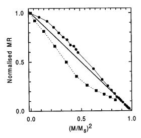
FIG. 14. Normalized anhysteretic magnetoresistance versus reduced magnetization for a dipolar sample (squares) and for a non-interacting sample (circles). Parameters: p = 30% (Co<sub>16</sub>Cu<sub>84</sub>) and T = 82 K. Coalescence is allowed in both samples.
