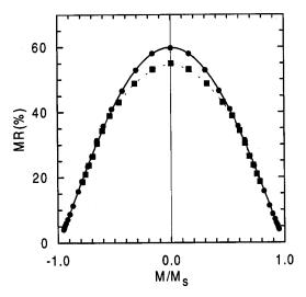
FIG. 6. Anhysteretic magnetoresistance versus reduced sample magnetization for a dipolar sample (squares) and for a noninteracting sample (circles). Parameters: p = 30% (Co<sub>16</sub>Cu<sub>84</sub>) and T = 82 K. Monodisperse samples.
