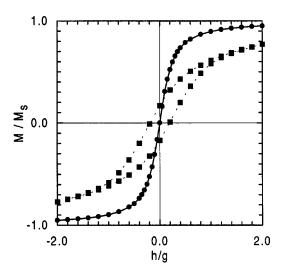
FIG. 2. Hysteresis loop for a dipolar system (squares) and magnetization curve for a noninteracting system (circles). Parameters p = 30% (Co<sub>16</sub>Cu<sub>84</sub>) and T = 82 K. Monodisperse samples.
