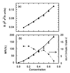
FIG. 7. Concentration dependence of (a) the zero-field resistance and (b) the zero-field magnetoresistance of dipolar (squares) and noninteracting (circles) monodisperse  $\text{Co}_x\text{Cu}_{1-x}$  samples. The percentage change of the MR due to dipolar interactions is also shown (stars) and MR(ni), MR(i) denote the MR values for the noninteracting and interacting systems, respectively. Parameters: T=8~K.
