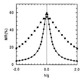
FIG. 5. Field dependence of anhysteretic magnetoresistance for a dipolar sample (squares) and for a noninteracting sample (circles). Parameters: p = 30% (Co<sub>16</sub>Cu<sub>84</sub>) and T = 82 K. Monodisperse samples.
