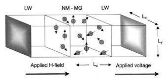
FIG. 1. Sketch of the geometry used to calculate the conductivity of the granular alloy.
