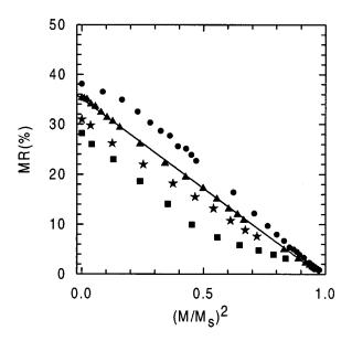
FIG. 13. Anhysteretic magnetoresistance versus reduced magnetization. Data for a monodisperse noninteracting system (triangles), a monodisperse dipolar system (stars), a polydisperse noninteracting system (circles), and a polydisperse dipolar system (squares) are shown. The monodisperse samples have V=3 and the polydisperse samples have  $\langle V \rangle \sim 3.06$ . (The volume of a monomer is defined as the volume unit). Parameters: p=30% (Co<sub>16</sub>Cu<sub>84</sub>) and T=82 K.
