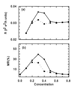
FIG. 10. Concentration dependence of (a) the zero-field resistance and (b) the zero-field magnetoresistance of dipolar (squares) and noninteracting (circles)  $Co_xCu_{1-x}$  samples. Coalescence is allowed in all samples. Parameters: T = 82 K.
