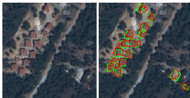
Fig. 1. Automated building detection from very high resolution multispectral data. The developed algorithm managed to detect efficiently scene's buildings. The ground truth data are shown with a green color, while the detected buildings with red.
