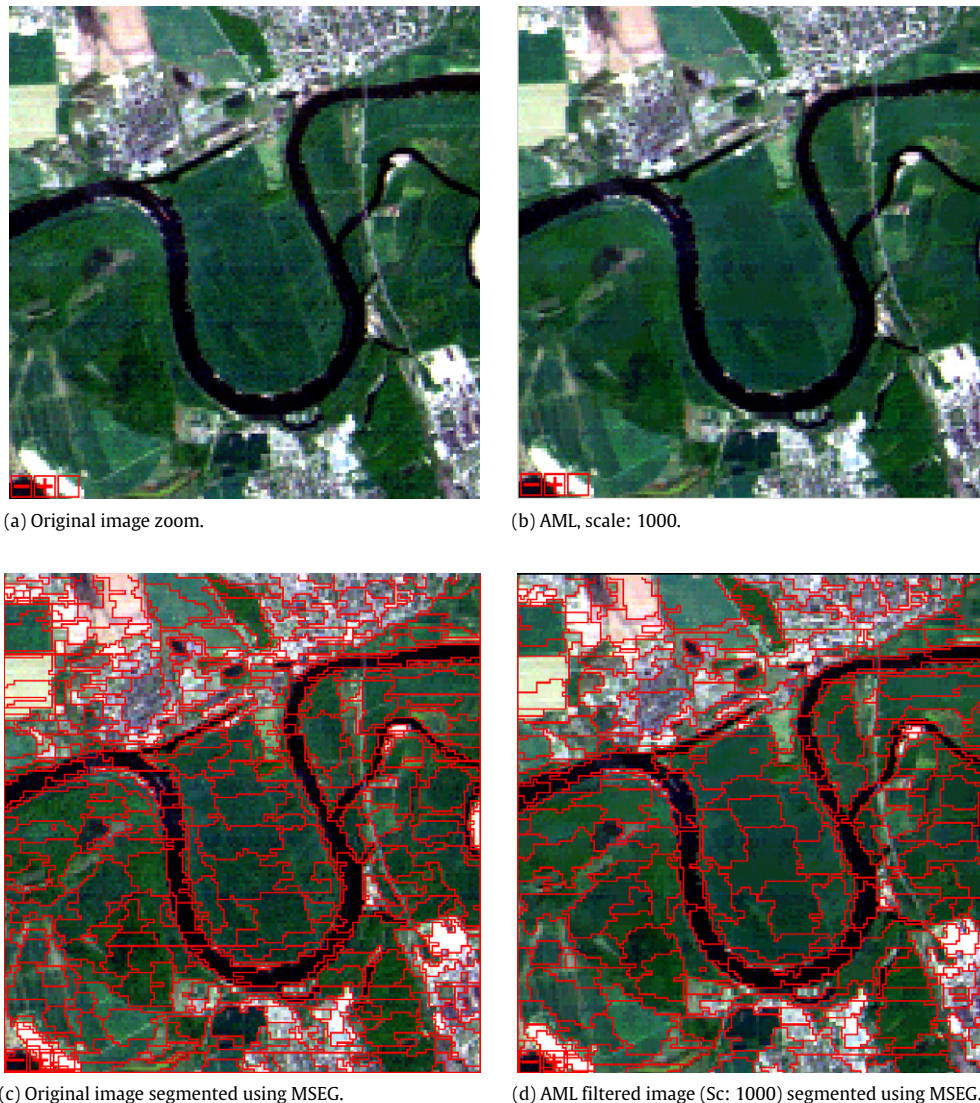
Fig. 8. A segmentation test as performed on a Landsat TM image, with and without the application of nonlinear filtering.
