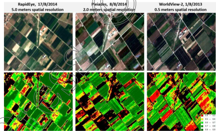
Fig. 6 Canopy greenness estimation on the Vegora agricultural region from different satellite sensors (i.e., RapidEye, Pleiades, WorldView-2) and spatial resolutions. The natural color composites are shown in the top and the estimated canopy greenness levels from the developed system, on the bottom.
