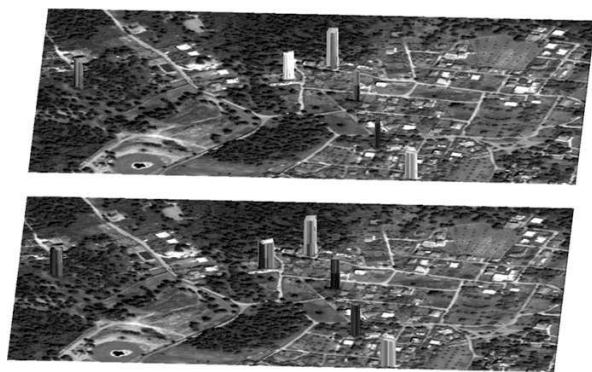
Fig. 4 The detected changes (new buildings) in 3D after the application of the unsupervised change detection procedure on QuickBird 2007 and 2009 satellite data. The detected new building in 3D are shown in the upper part, while the 3D buildings from the ground truth data are shown in the bottom. After a close inspection one can observe the low completeness and high correctness detection rates of the unsupervised change detection algorithm
