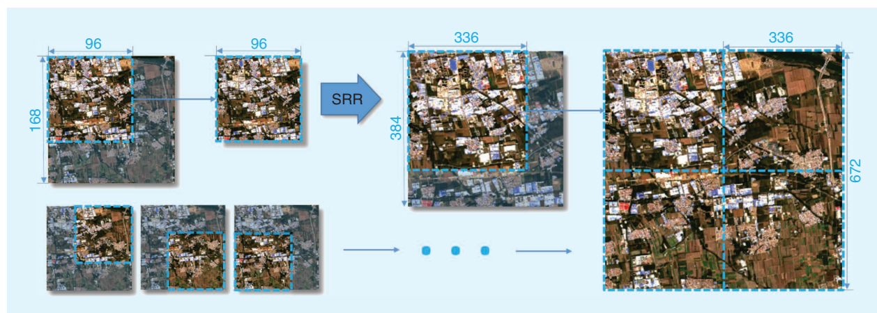
FIGURE 28. An example of the clipping-and-merging method pipeline. The input image has a size of 168 \times 168 and is cropped into four overlapping patches, each with a size of 96 \times 96 . The patches are independently downscaled by an SR algorithm (denoted SRR here), producing four 384 \times 384 images. Half of the overlap region of each patch is then clipped, ending up with four 336 \times 336 images, which are then joined to produce the final SR prediction. (Source: [206]; used with permission.)
