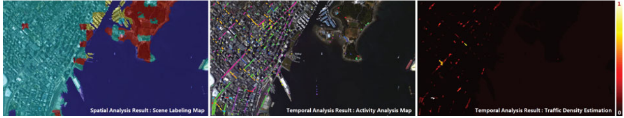
Fig. 12. Final results. From left to right: spatial scene labeling (cyan, red, yellow, and blue represent urban, vegetative cover, harbour, and river, respectively.), temporal activity analysis (each color corresponds to a cluster), and traffic density estimation (from [39]).
