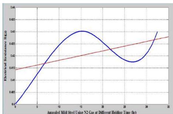
Fig. 7. Effect of annealing using N 2 gas at different holding time on the electrical resistance
