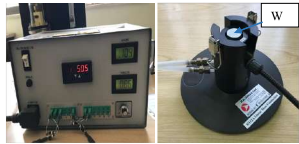
Fig. 2. H112A Linear heat conduction instrument (Hilton Type) used to investigate the thermal conductivity
