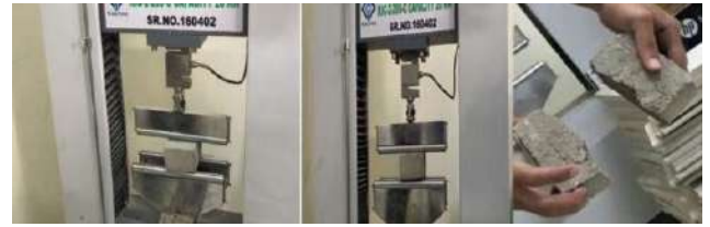
Fig.3. Testing the Bricks by Universal Testing Machine
