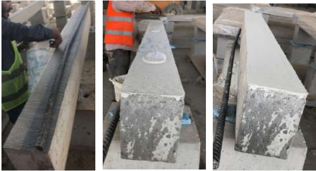
Fig. 5. Installation of external textile fabric
