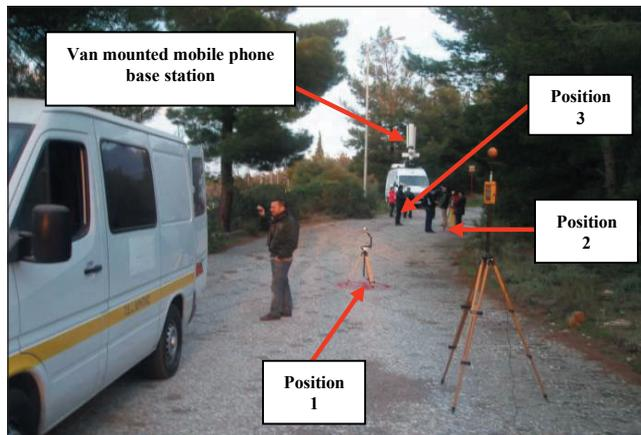
Fig. 4. The mobile phone base station and the measurement positions in the area of the N.C.S.R. “Demokritos” (measurement scenarios 1 and 2).
