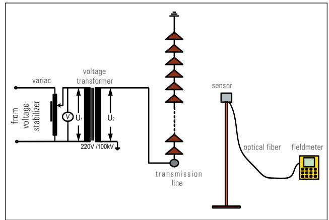
Fig. 1. Test setup for the measurement of the Electric Field (E).
