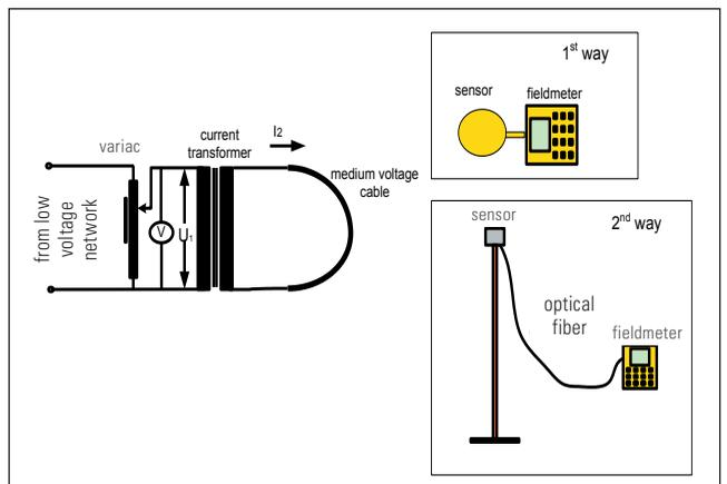
Fig. 2. Test setup for the measurement of the Magnetic Field (B),
