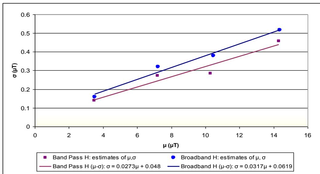
**Figure 8: Variation ( $\mu$ - $\sigma$ ) for the measurements of Magnetic Field (B)**
