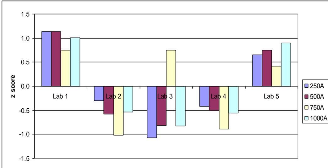
Figure 6: Z-scores for broadband measurements of Magnetic Field (B)
