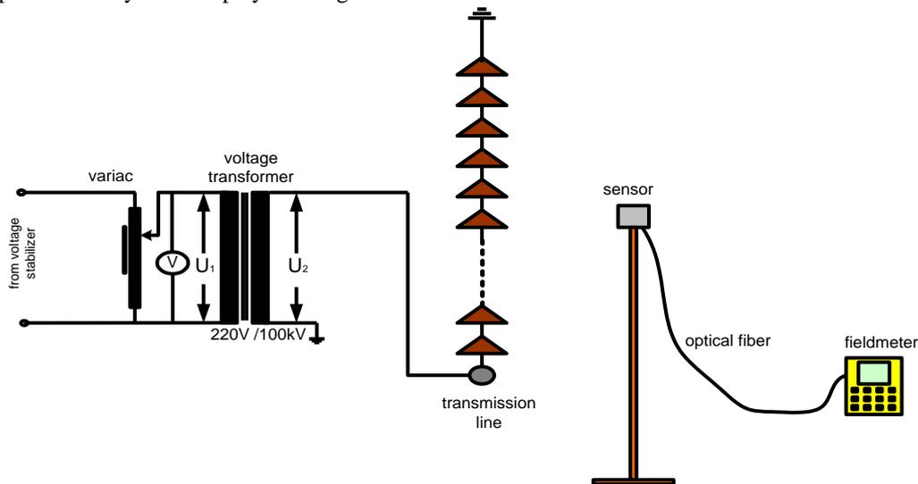
**Figure 1: Test setup for the measurement of Electric Field (E)**
