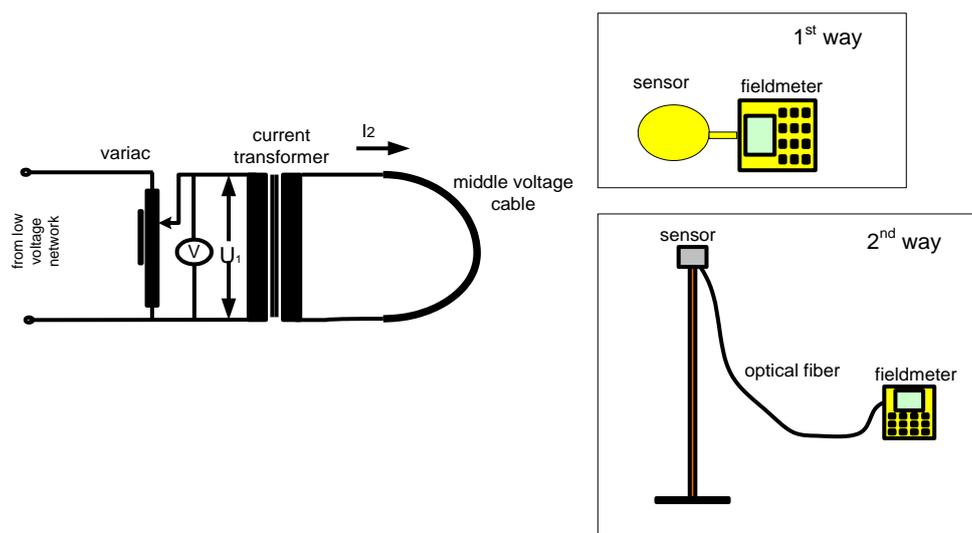
**Figure 2: Test setup for the measurement of Magnetic Field (B)**
