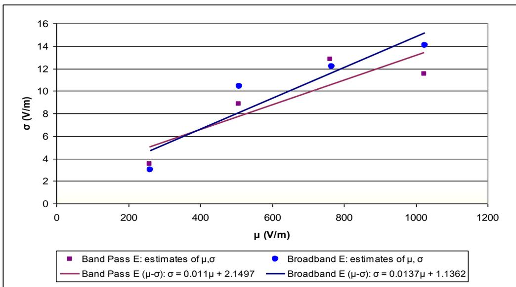
Figure 7: Variation ( $\mu$ - $\sigma$ ) for the measurements of Electric Field (E)
