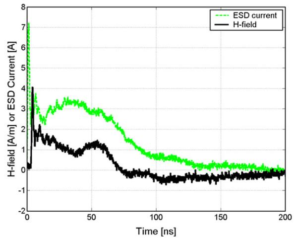
Fig. 4. ESD current and  $H$ -field for the NSG-438 ESD generator at 20 cm from the discharge point, in direction  $A$  (charging voltage = +2 kV).
