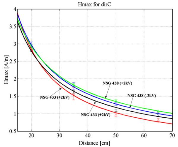
Fig. 7. Peak of  $H$ -field for various distances from the discharge point in direction  $C$ , using the NSG-433 and NSG-438 ESD generators.
