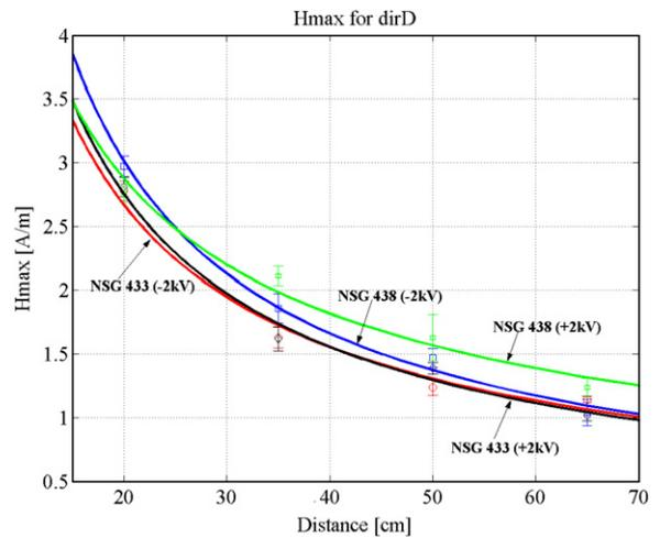
Fig. 8. Peak of  $H$ -field for various distances from the discharge point in direction  $D$ , using the NSG-433 and NSG-438 ESD generators.
