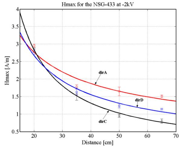
Fig. 11. Peak of magnetic field strength for the NSG-433 ESD generator for three perpendicular directions on the horizontal plane (charging voltage = -2 kV).
