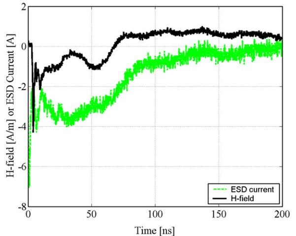
Fig. 5. ESD current and  $H$ -field for the NSG-438 ESD generator at 20 cm from the discharge point, in direction  $A$  (charging voltage = -2 kV).
