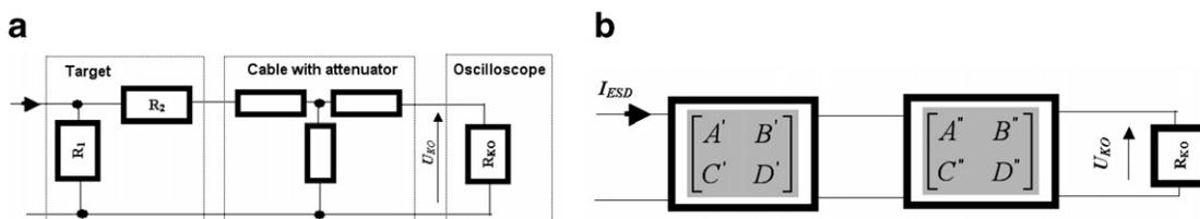
Fig. 3. The equivalent circuit of the ESD generator at DC analysis.
