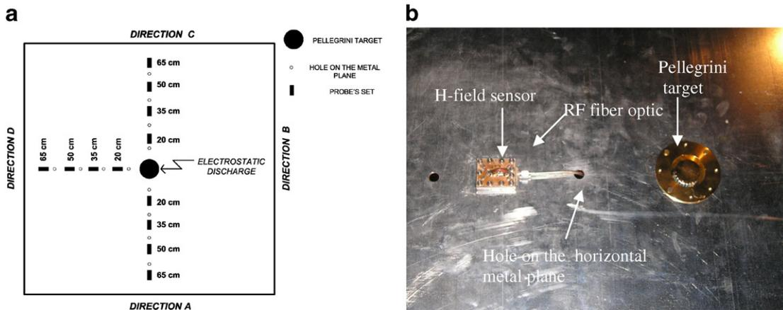
Fig. 2. (a) The measurement points where the *H*-field sensor was placed. (b) Position of the *H*-field sensor on the grounded metal plane.
