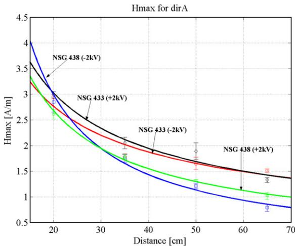
Fig. 6. Peak of  $H$ -field for various distances from the discharge point in direction  $A$ , using the NSG-433 and NSG-438 ESD generators.
