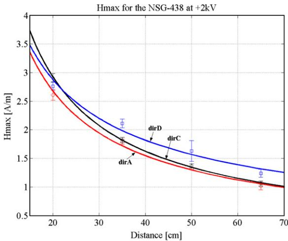
Fig. 10. Peak of magnetic field strength for the NSG-438 ESD generator for three perpendicular directions on the horizontal plane (charging voltage = +2 kV).
