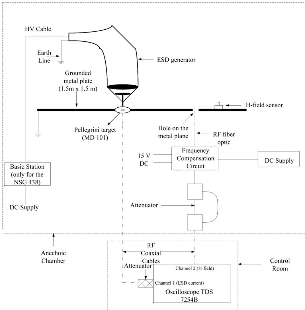
Fig. 1. Experimental set-up.
