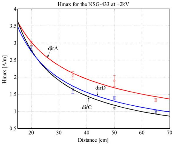
Fig. 9. Peak of magnetic field strength for the NSG-433 ESD generator for three perpendicular directions on the horizontal plane (charging voltage = +2 kV).
