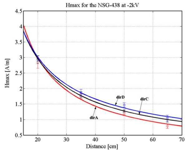
Fig. 12. Peak of magnetic field strength for the NSG-438 ESD generator for three perpendicular directions on the horizontal plane (charging voltage = -2 kV).
