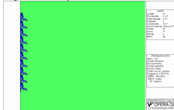
Fig. 2: Two dimensional model of the insulator string.
