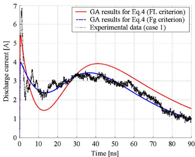
**Figure 13.** Curve comparison between the experimental data of the discharge current and the discharge current for the optimized parameter values of equation (4) for the first case and for different error criteria.
