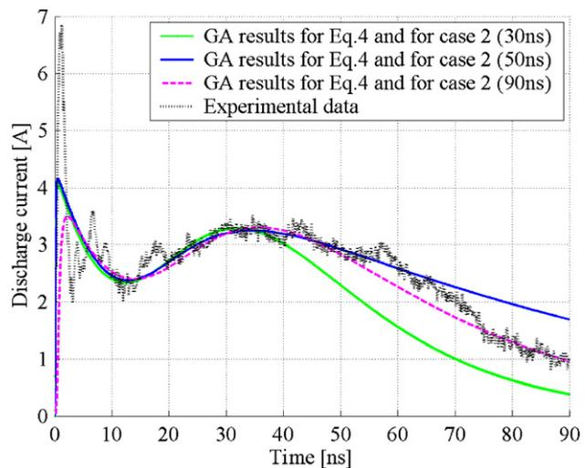
**Figure 11.** Curve comparison between the experimental data of the discharge current and the discharge current for the optimized parameter values of equation (4) for the second case and for different time durations.
