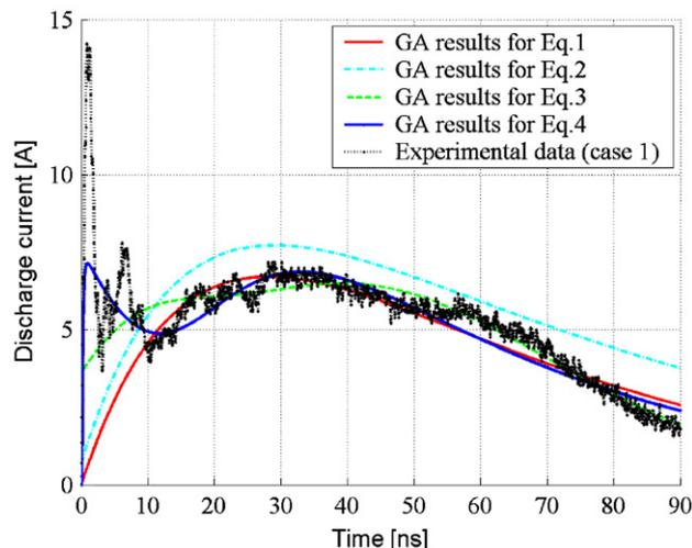
**Figure 7.** Curve comparison between the experimental data of the discharge current and the discharge current for the optimized parameter values of (1)–(4) for the first case (charging voltage = +4 kV).
