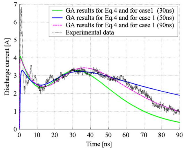
**Figure 10.** Curve comparison between the experimental data of the discharge current and the discharge current for the optimized parameter values of equation (4) for the first case and for different time durations.
