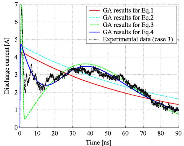
**Figure 6.** Curve comparison between the experimental data of the discharge current and the discharge current for the optimized parameter values of (1)–(4) for the third case (charging voltage = +2 kV).
