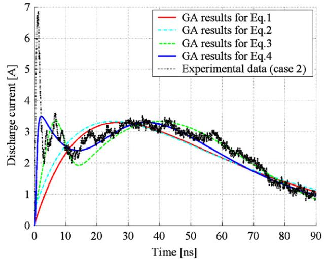
**Figure 5.** Curve comparison between the experimental data of the discharge current and the discharge current for the optimized parameter values of (1)–(4) for the second case (charging voltage = +2 kV).
