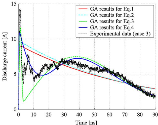
**Figure 9.** Curve comparison between the experimental data of the discharge current and the discharge current for the optimized parameter values of (1)–(4) for the third case (charging voltage = +4 kV).
