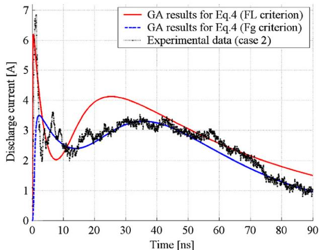
**Figure 14.** Curve comparison between the experimental data of the discharge current and the discharge current for the optimized parameter values of equation (4) for the second case and for different error criteria.
