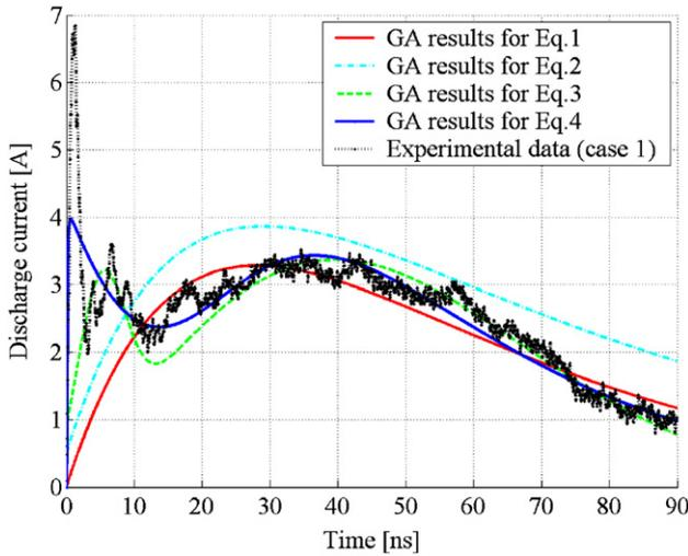
**Figure 4.** Curve comparison between the experimental data of the discharge current and the discharge current for the optimized parameter values of (1)–(4) for the first case (charging voltage = +2 kV).
