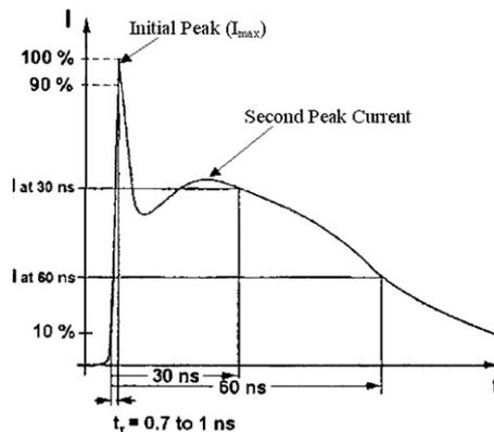
Figure 1. Typical waveform of the output current of the ESD generator [1].
