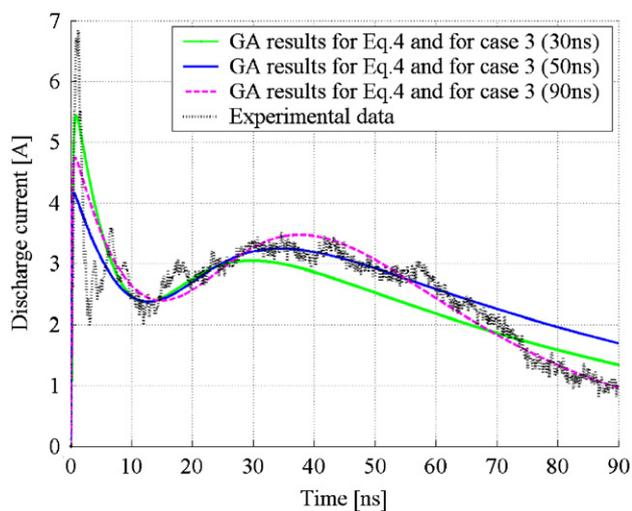
**Figure 12.** Curve comparison between the experimental data of the discharge current and the discharge current for the optimized parameter values of equation (4) for the third case and for different time durations.
