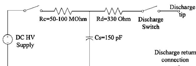
Figure 2. Simplified diagram of the ESD generator [1].
