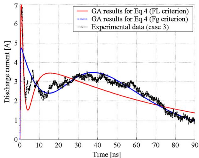
**Figure 15.** Curve comparison between the experimental data of the discharge current and the discharge current for the optimized parameter values of equation (4) for the third case and for different error criteria.
