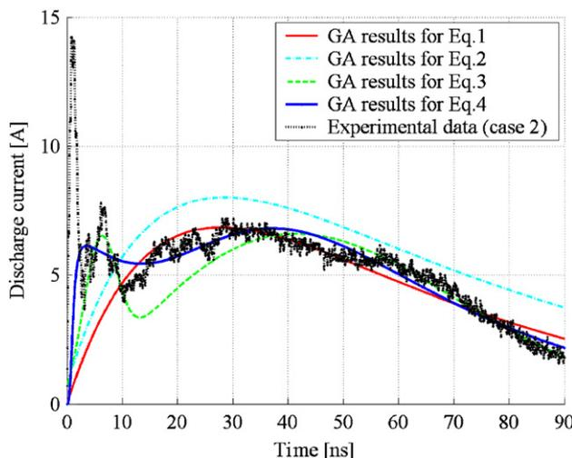
**Figure 8.** Curve comparison between the experimental data of the discharge current and the discharge current for the optimized parameter values of (1)–(4) for the second case (charging voltage = +4 kV).
