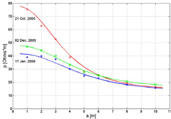
Fig. 1. Variation of the apparent soil resistivity in relation to the distance of the auxiliary electrodes in three different days.
