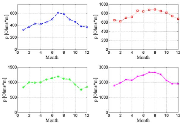
Fig. 2. Variation of the apparent soil resistivity during the year at various areas ( $a=10m$ ).
