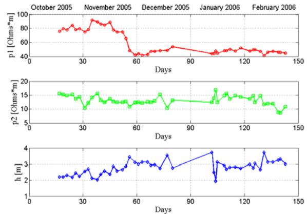
Fig. 5. Variation of two-layer earth parameters during the year.
