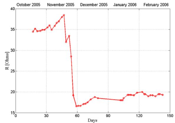
Fig. 6. Variation of grounding system resistance during the year.
