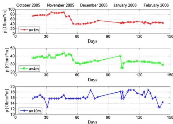
Fig. 4. Variation of the apparent soil resistivity upon the distance of the auxiliary electrodes ( $a=1\text{m}$ ,  $a=4\text{m}$  and  $a=10\text{m}$ ).
