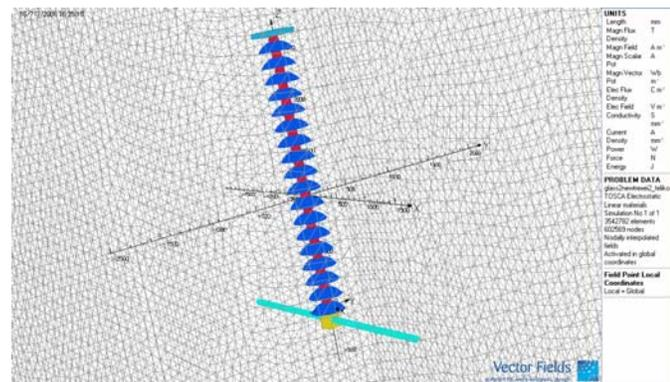
Fig. 3. The three dimensional model of the glass insulator string.
