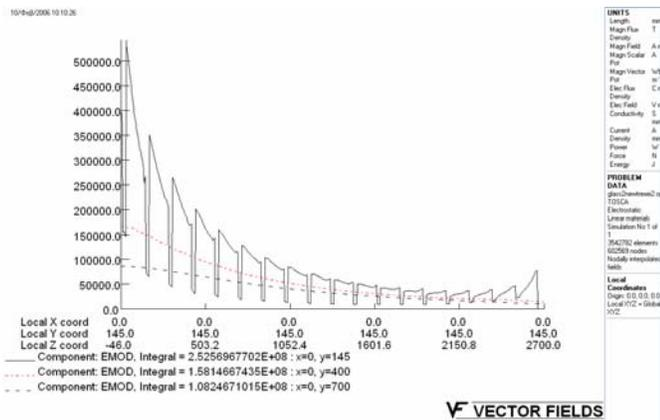
Fig. 9. Electric field along lines parallel to the glass insulator string and vertical to the Y-axis.
