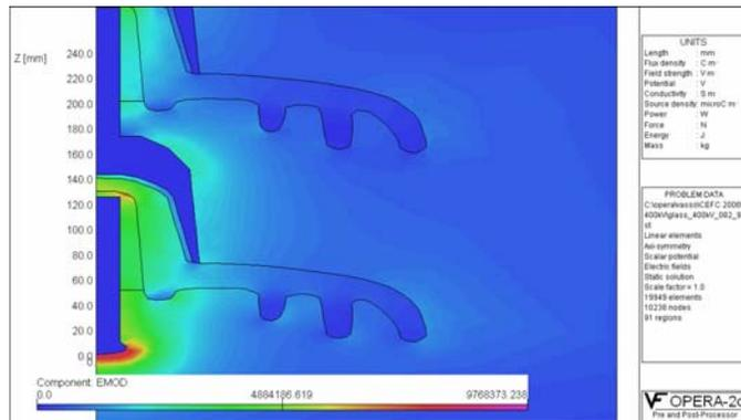
Fig. 2. Electric field contours of a part of the glass insulator string.
