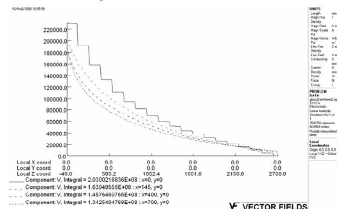
Fig. 6. Potential along lines parallel to the glass insulator string and vertical to the conductor (X-axis).
