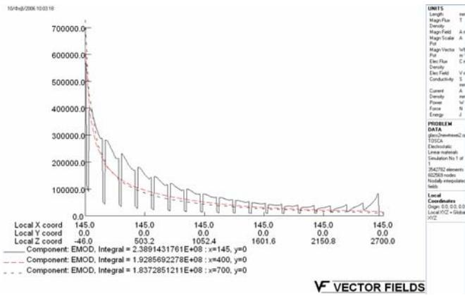
Fig. 7. Electric field along lines parallel to the glass insulator string and vertical to the conductor (X-axis).
