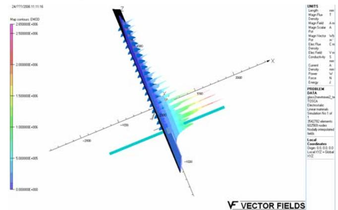
Fig. 5. Histogram of the electric field in a cartesian patch on YZ plane of the glass insulator string.
