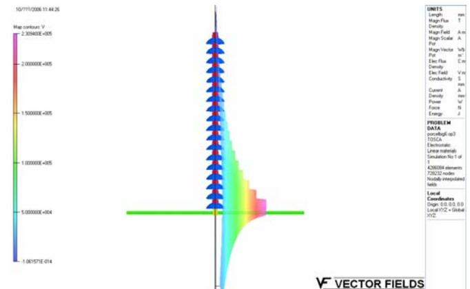
Fig. 10. Histogram of the potential in a cartesian patch on YZ plane of the porcelain insulator string.
