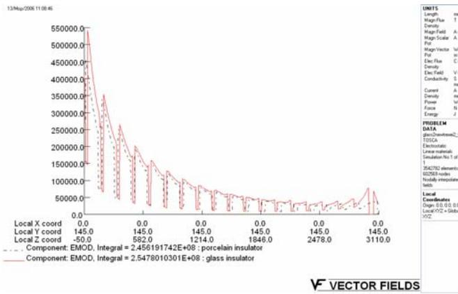
Fig. 13. Electric field along porcelain and glass insulator string.
