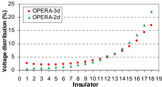
Fig. 14. Comparison between two and three dimensional models of the glass insulator string.
