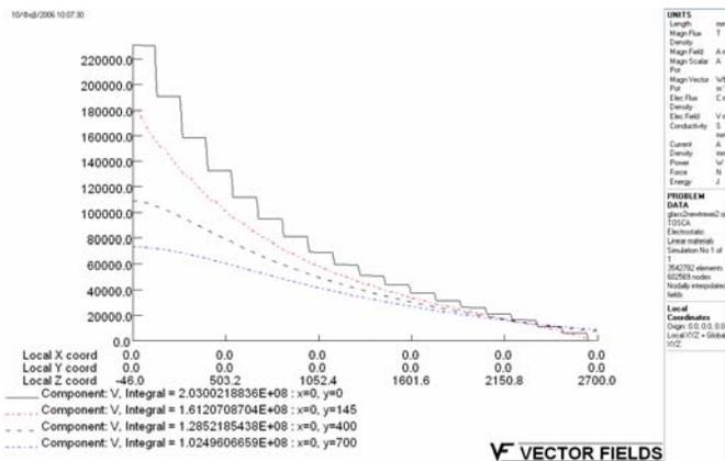
Fig. 8. Potential along lines parallel to the glass insulator string and vertical to the Y-axis.
