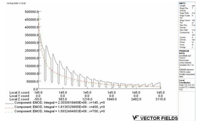
Fig. 11. Electric field along lines parallel to the porcelain insulator string and vertical in the X-axis.
