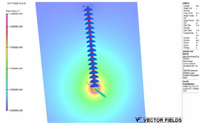
Fig. 4. Potential distribution of the glass insulator string.
