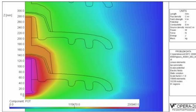
Fig. 1. Potential contours of a part of the glass insulator string.
