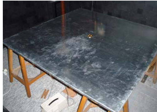
Fig.3: Target mounted on the horizontal metal plane with dimensions 1.5\text{ m} \times 1.5\text{ m} (case 1).
