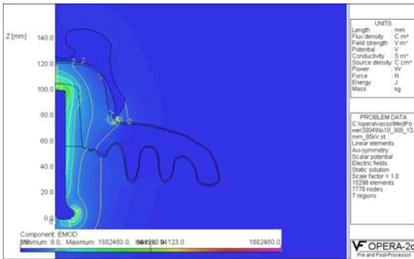
Figure 7: Electric field around and inside of a heavily polluted insulator.
