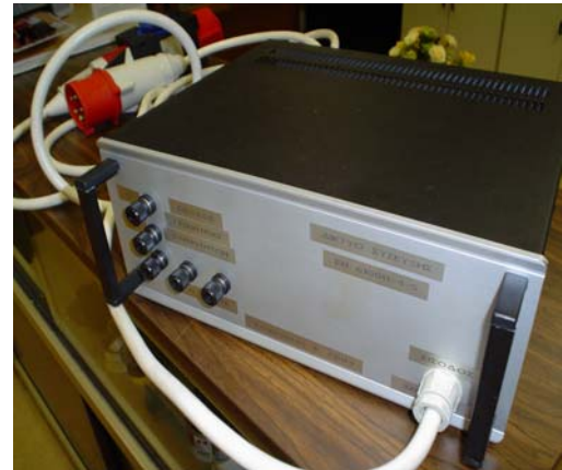
Figure 17: The constructed 3-phase coupling network
