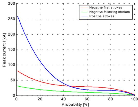
Figure 2. Lightning current peak value distribution
