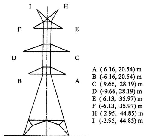
Figure 5: Typical tower of the analyzed 400kV Hellenic transmission line
