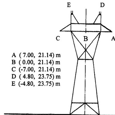
Figure 4: Typical tower of the analyzed 150kV Hellenic transmission line
