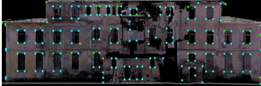
Fig. 7. Residuals between the points obtained from MS and classic methods
