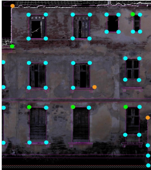
Fig. 8. Check points with higher residual values (orange color)
