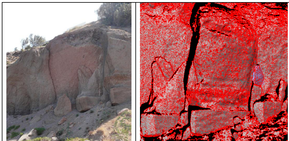
Figure 3. Point cloud of the area showing some of the unstable rocks and the developed tension cracks in detail.
