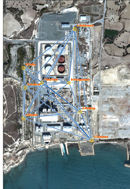
Figure 1 Plan of the network as designed and implemented depicting the control points
