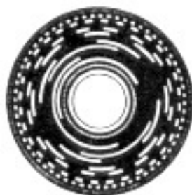
Fot.2. Code-circle of the digital theodolites
