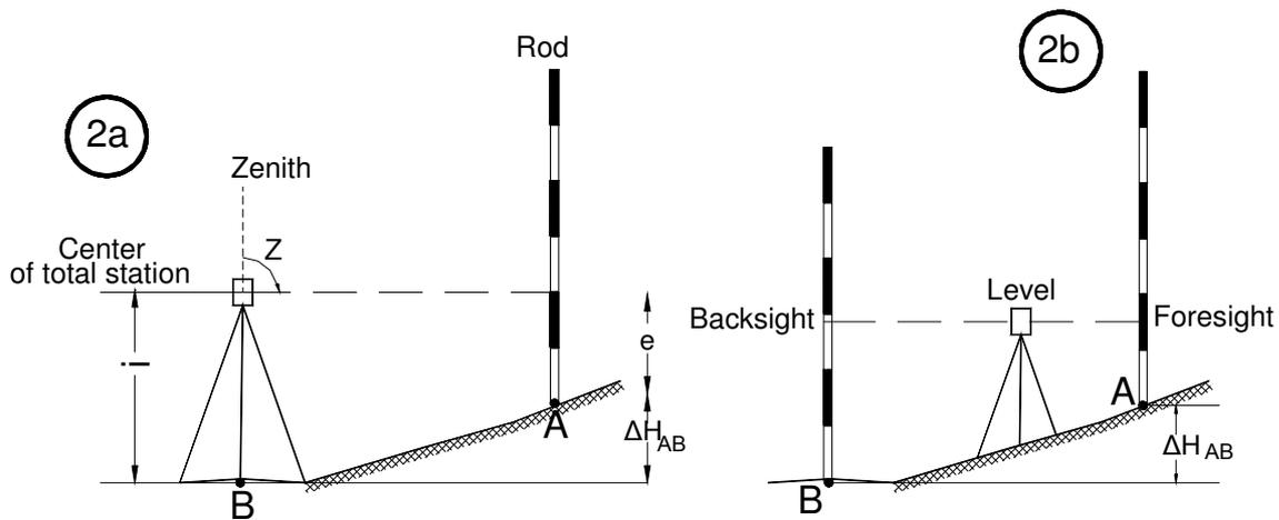
Figure 2. Accurate determination of the instrument's height.
