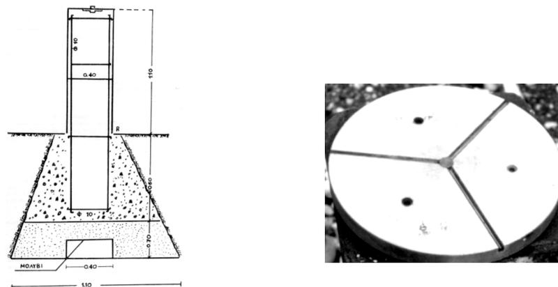
Fot.1: The marking of the points of the 3d standard geodetic network.
