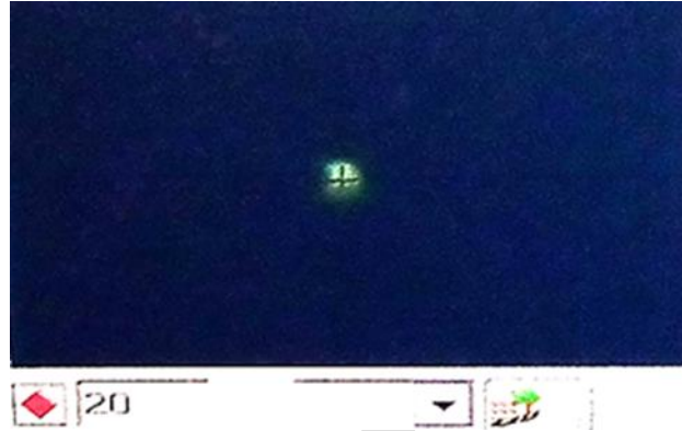
Figure 8. Aiming at the Polaris with Wireless Remote Survey method via the screen of the “User Device” [14]
