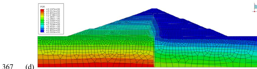
368 **Figure 7. Finite-element analysis of the dam: (a) FE mesh (dimensions in metres), (b) dam displacements, (c)**
